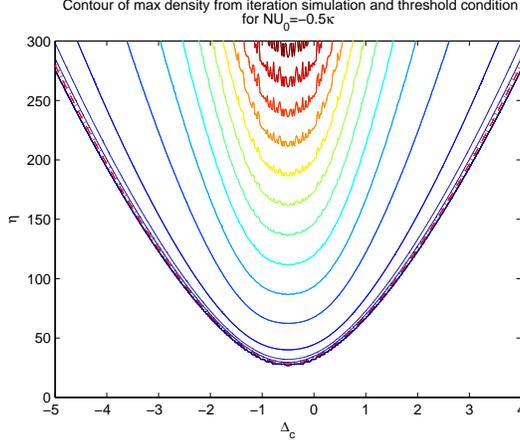
Fig. 1. Contour lines of the maximum of the selfconsistent atom density distribution for a cloud at rest as a function of detuning  $\delta_c$  and pump amplitude  $\eta$ . The analytic formula for the selforganization threshold is indicated by the red dashed line. Parameters are  $N = 200, U_0 = -1/400, \kappa = 1$ .
